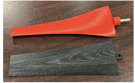
Figure 2: Evolution of blade prototypes from PLA (bottom) to final ABS (top).
