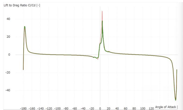
Figure 1: Polar analysis of the A18 airfoil showing lift-to-drag ratio.
