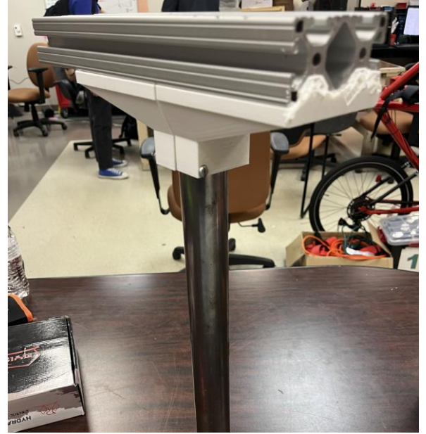
Figure 4: Picture of Stanchion holding Aluminum Rail and Tower Together
